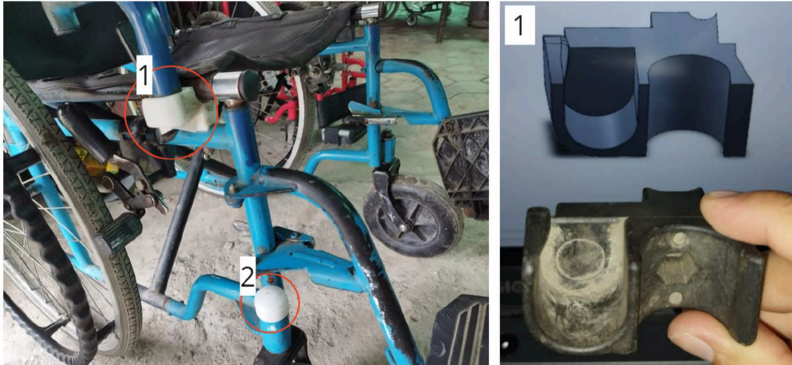
Figure 10 Wheelchair components (1) CAD model prepared for 3D printing (Upper) and original damaged seat clamp sample (Lower) (2) 3d printed ring cap
