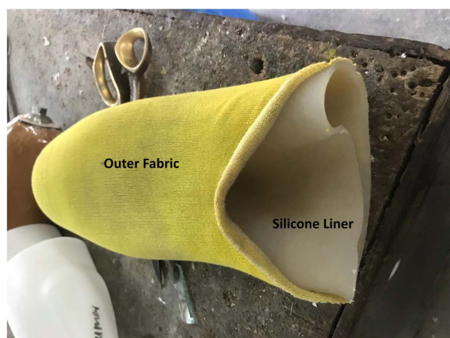
Figure 3. Common failure mode: detachment of the outer fabric.
