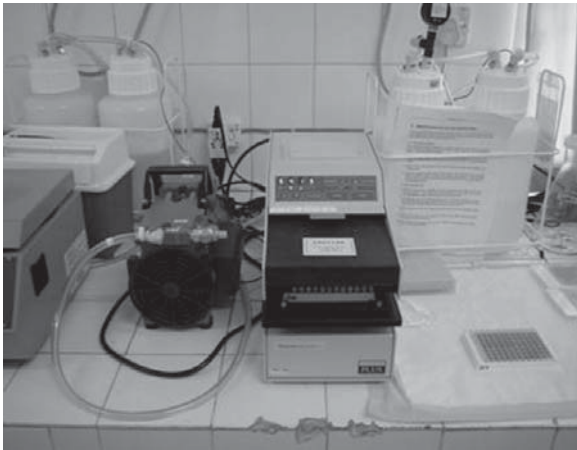
Figure 1b. An automated reader gives a measurement of optical density (presence of color) for each well
